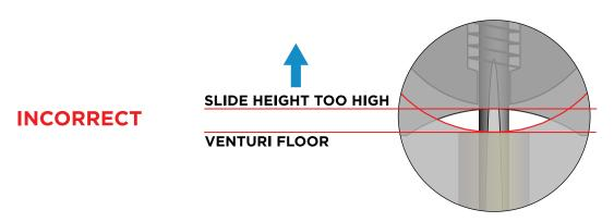
**Solution:** The proper tuning method would be to adjust the Clicker leaner until the idle RPMs begin to raise slightly. A small **Idle Set Screw** adjustment may still be necessary to dial in the idle RPMs, but the slide cutaway height would likely now remain near 1.8mm and the user would not have any hard starting issues resulting from a slide cutaway height that is too high.
