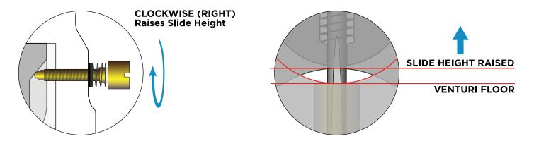
Turning the screw out counterclockwise to the left will lower the slide height:
