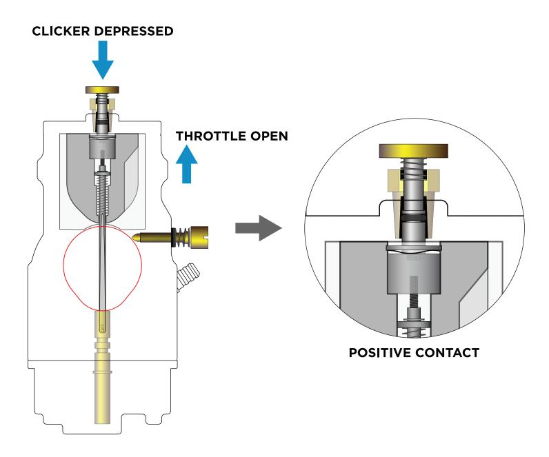
Adjusting the **Clicker Adjuster** to the right, or clockwise, will raise the metering rod within the slide. Raising the metering rod will add more fuel to the mixture as it exposes more of the angled surface grind of the metering rod at the top of the nozzle near the venturi floor.
