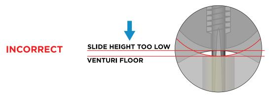
**Solution:** The proper tuning method would be to adjust the **Clicker** a bit richer, one or two clicks at a time richer until the idle RPMs come down slightly. From there a small adjustment may still be necessary to the **Idle Set Screw** to fine tune the idle RPMs, but the slide cutaway height would likely remain close to 1.8mm and the user would not experience issues related to a slide cutaway height that is too low.
