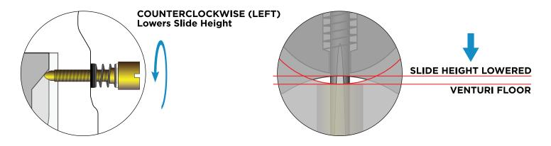
**NOTE:** If turning the screw out does not lower the slide height, the slide may be hung up on the throttle cable and a throttle cable length adjustment may be necessary.
